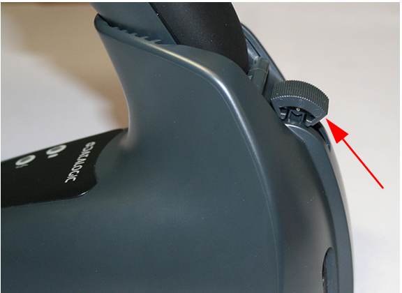
Figure 2. Lever in locked position
